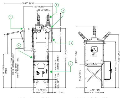
Side View at Maximum Height (Dimensions given for support at min/max height) Front View at Maximum Height (Dimensions given for support at min/max height)
