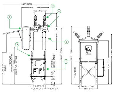
Side View at Maximum Height (Dimensions given for support at min/max height)
